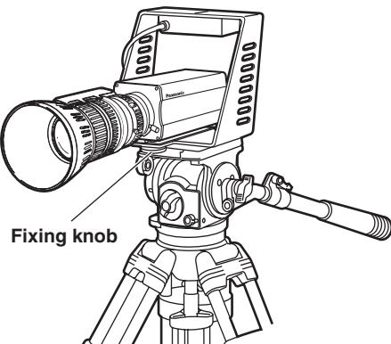
4 Slide the viewfinder onto the mounting base and tighten the fixing knob to secure it firmly.
