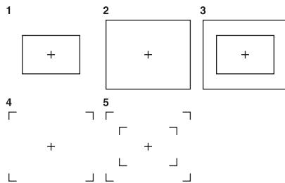
The inner frame and the outer frame are approximately 90% and 95%, respectively, of the safety zone.
